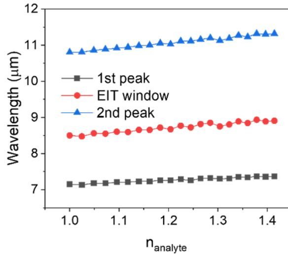
**Fig. 7.** The peak position of the first reflection peak, the middle of the EIT window, and the second reflection peak as a function of simulated analyte refractive index.
