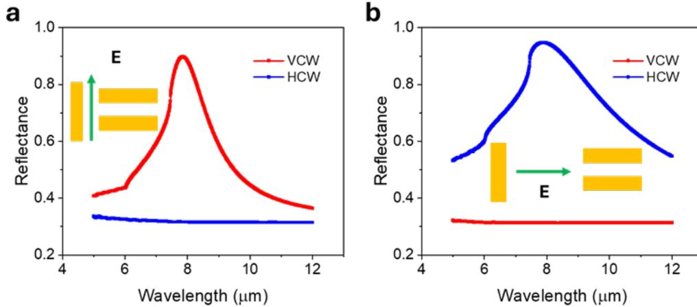
**Fig. 2.** (Color online) Simulated reflectance spectra of separated VCW (red) and HCW (blue) metamaterials at (a) the TE mode and (b) the TM mode at normal incident.
