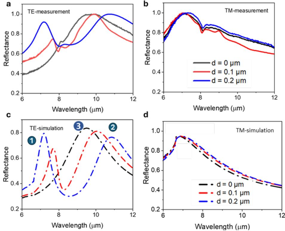
**Fig. 3.** (Color online) (a-b) Measured and (c-d) simulated reflectance of the EIT structure with different levels of asymmetry, with  $d = 0 \mu\text{m}$  (black),  $d = 0.1 \mu\text{m}$  (red), and  $d = 0.2 \mu\text{m}$  (blue) curves. The studied polarizations are TE and TM, as mentioned inside each figure panel, with the electric field polarizations pointing toward the VCW and HCW, respectively. The incident angles are  $15^\circ$  for the measurements and  $0^\circ$  for simulations.
