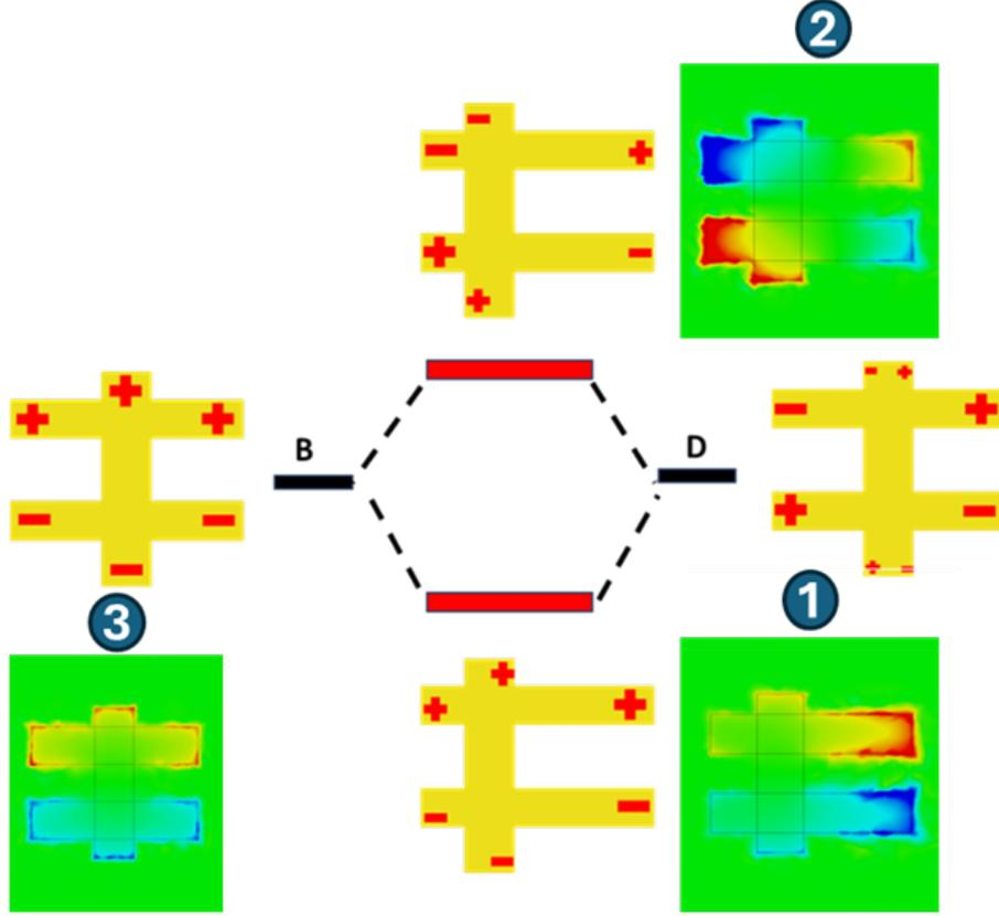
**Fig. 5.** Simulated electric field distributions at different resonant frequencies according to spectral positions (1), (2), and (3), corresponding to the wavelengths of  $7 \mu\text{m}$ ,  $10.8 \mu\text{m}$ , and  $9.6 \mu\text{m}$ , respectively, in Fig. 3c.
