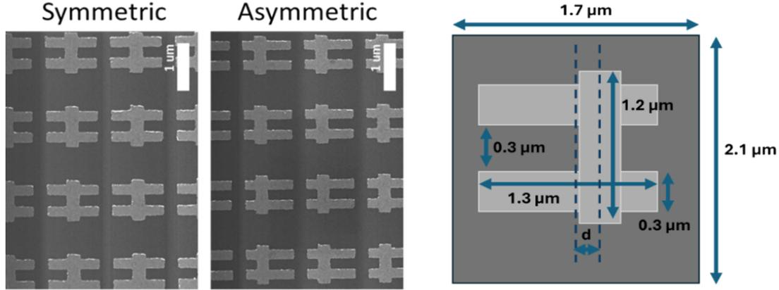
**Fig. 1.** SEM images of symmetric and asymmetric metamaterial samples and a sketch of the symmetric unit cell with the lateral displacement denoted as  $d$ .
