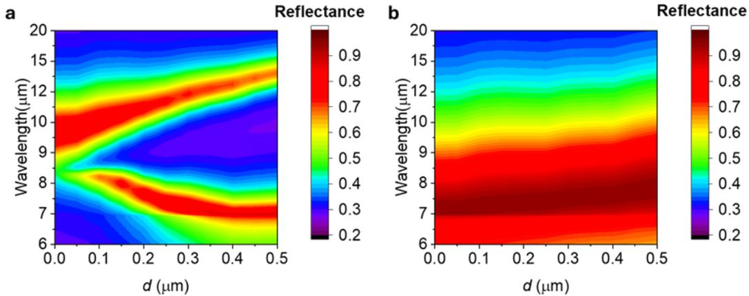
**Fig. 4.** (Color online) Extended simulation on reflectance of EIT metamaterials as function of  $d$ , varying from 0 to  $0.5 \mu\text{m}$  for (a) TE mode and (b) TM mode.
