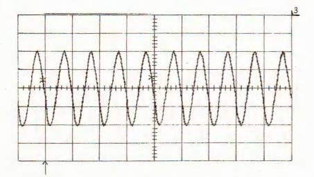
Amplitude at point (3) after balancing at n = 3000 rpm
