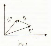
The unit of  $\overline{\alpha}_{jk}$  is [m/kg] or [mm/g]. By changing the test weights at the balancing plane k (k = 1, ..., K) we will determine the influence coefficients  $\overline{\alpha}_{jk}$  (j = 1, ..., J), (k = 1, ..., K).
