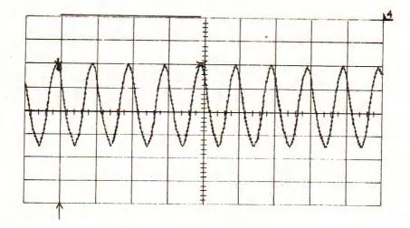
Amplitude at point (4) before balancing at n = 3000 rpm
