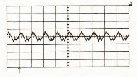
Amplitude at point (2) after balancing at n = 3000 rpm
