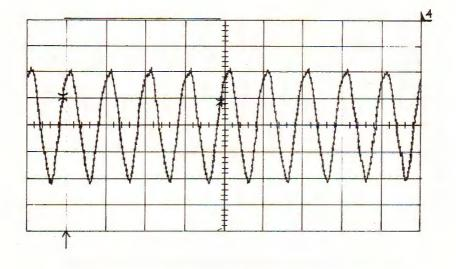
Amplitude at point (4) after balancing at n = 3000 rpm
