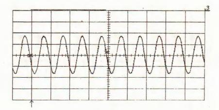
Amplitude at point (3) before balancing at n = 3000 rpm
