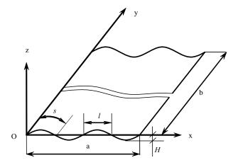
Fig. 1. Model of a corrugated plate
