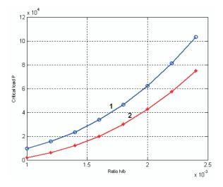
Fig. 2. Effect of plate thickness on buckling load 1. Seydel's technique, 2. Proposed approach
