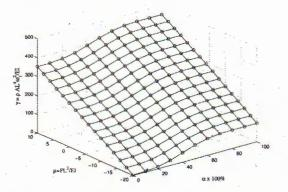
Fig. 9. Frequency parameter of partially supported CS beams at various values of axial force parameter and supporting percentages ( $k_0 = 100$ )
