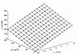
Fig. 5. Influence of axial force and foundation stiffness on frequency parameter of fully supported CS beam
