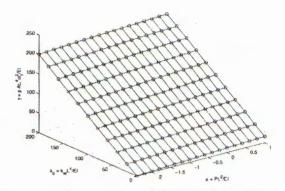
*Fig. 4.* Influence of axial force and foundation stiffness on frequency parameter of fully supported CF beam
