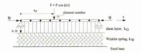
Fig. 2. Simply supported prestressed beam resting on a two-parameter elastic foundation foundation subjected to a moving harmonic load  $F = P\cos(\Omega t)$
