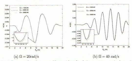
Fig. 4. Response of simply supported beam without foundation support to moving harmonic load at various values of axial force and at a velocity  $v=20\,m/s$
