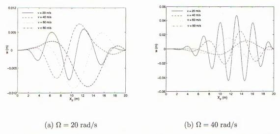
Fig. 5. Response of simply supported beam without foundation support to moving harmonic load with various velocities and at an axial force  $Q = -2000 \, kN$
