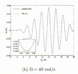
Fig. 3. Deflection under the moving load for constant velocity  $v = 15 \, m/s$  and at different excitation frequencies
