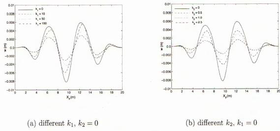
Fig. 6. Response of simply supported beam without foundation support to moving harmonic load at different values of foundation parameters and at  $v = 20 \, m/s$ ,  $\Omega = 20 \, rad/s$ ,  $Q = -2000 \, kN$
