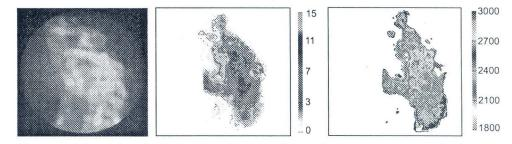
*Fig.* 4. Picture of flame by visioscope, distribution of soot fraction and temperature given by the two-color method (60% load, n=2000 rpm, 9<sup>0</sup> CA)
