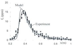
Fig. 6. Comparing soot fraction given by model and by experiment (Re=31.020)
