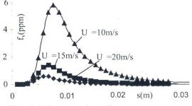
Fig. 2. Influence of gas flow movement rate on soot fraction in the combustion chamber  $\theta = \frac{\pi}{4}$
