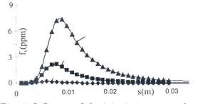
Fig. 1. Influence of the injection spray angle on soot fraction in the combustion chamber (gas flow movement rate  $U_{\infty} = 4$  m/s)
