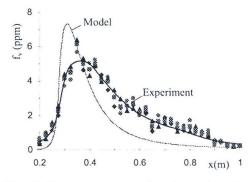
Fig. 5. Comparing soot fractions given by model and by experiment (Re=23.180)
