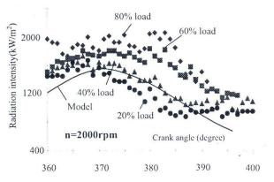
Fig. 11. Comparison of variations in radiation intensity from the flame to the auxiliary chamber wall of Mazda engine in relation to Crank angle corresponding to different load regimes (n=2000 rpm)
