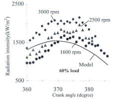
Fig. 10. Comparison of radiative heat transfer intensity from the flame to the combustion chamber wall at different engine speed regimes
