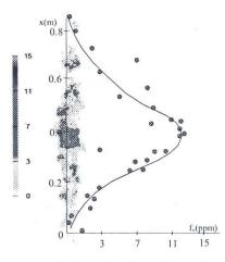
Fig. 3. Distribution of soot fraction according to the flame height given by the two-color method
