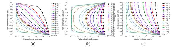
*Fig. 1.* Different profiles of FGM for several ranges of power law parameters (a) a = 1, b = 0 (classical profile) (b) a = b = 1, c = 2.0 (symmetric profile) (c) a = 1, b = 0.5, c = 2.0
