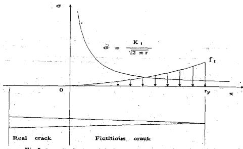
Fig. 2. Stress distribution and the fracture process some in front of a crack tip
