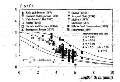
Fig. 4. Checking the size effect law by test and calculation data
