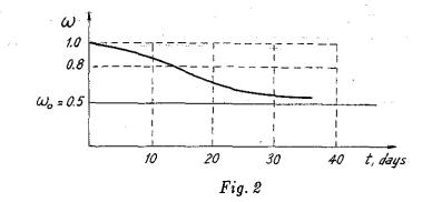
Consequently, if  $\omega < \omega_0$  the plate is stable for all the time, if  $\omega_0 < \omega$  the loss of stability is in determined time.  $\omega = \omega_0$  - the limit of long time stability,  $\omega_0 = 1 - \gamma$ .
