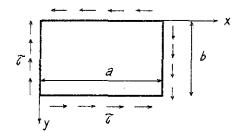
$$D\left(\frac{\partial^4 \Delta W}{\partial x^4} + 2\frac{\partial^4 \Delta W}{\partial x^2 \partial y^2} + \frac{\partial^4 \Delta W}{\partial y^4}\right) + 2N_{xy}\frac{\partial^2 \Delta W}{\partial x \partial y} = 0$$
