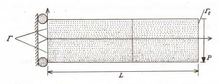
Fig. 1. A cantilever beam 2-D for comparison with the analytic solution from Timoshenko and Goodier
