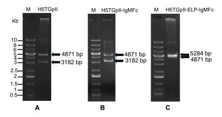
**Figure 2.** The electrophoresis image of the pCB301\_H5TGpII (A), pCB301\_H5TGpII-IgMFc (B) and pCB301\_H5TGpII-ELP-IgMFc (C) plasmids with the opposite expression being expressed for the gene coding for the kanamycin-resistant npt protein on themself vectors were cut by *Ncol* restriction enzyme. M: GeneRuler 1 kb Plus DNA Ladder (Fermentas).
