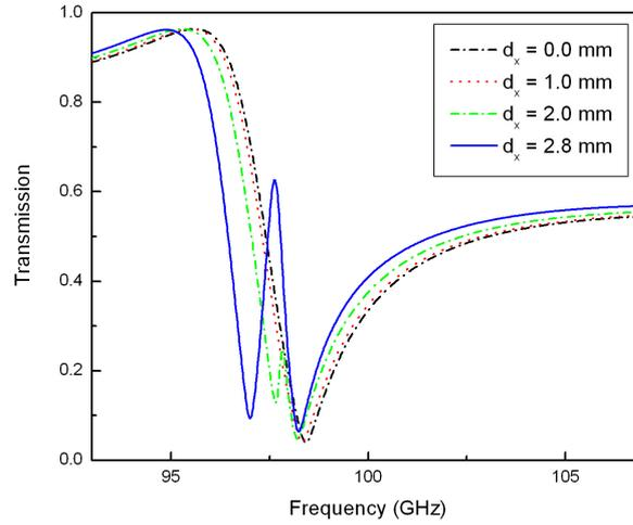
Figure 3. Transmission evolution of horizontally plasmon hybridized CWP super cell.
