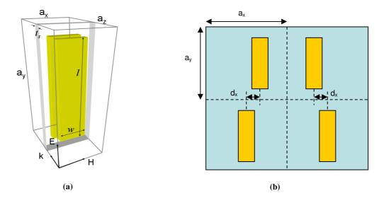
*Figure 1*. (a) A computational unit cell of CWP structure. (b) Schematic of a super cell CWP structure, including four original unit cells with the horizontal displacement d<sub>x</sub>.
