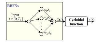
Figure 2. Radial Basis Function Neural Networks.
