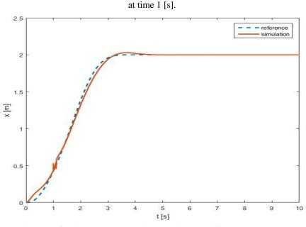
*Figure 8.* Trajectory of trolley when system is controlled by sliding mode controller combined with compensation anti-sway based on artificial neural network by PSO algorithm with the disturbance at time 1 [s].
