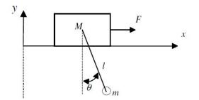
Figure 1. Overhead crane model.
