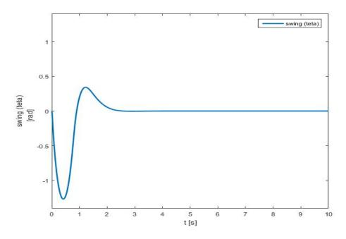
Figure 5. Swing angle of load when system is controlled by sliding mode controller without disturbance.
