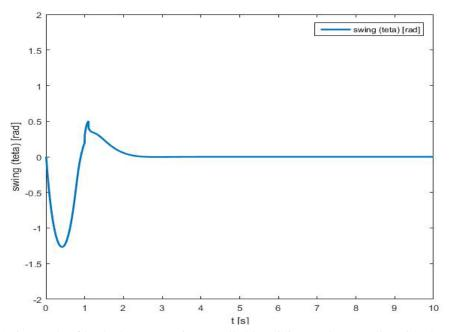
*Figure 7.* Swing angle of load when system is controlled by sliding mode controller with the disturbance
