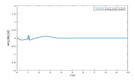
*Figure 9.* Swing angle of load when system is controlled by sliding mode controller combined with compensation anti-sway based on artificial neural network by PSO algorithm with the disturbance at time 1 [s].
