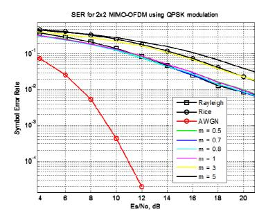
*Figure 7.* SER performance for 2×2 MIMO-OFDM system using QPSK modulation over different channels.
