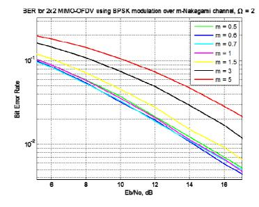
*Figure 4.* BER performance for 2×2 MIMO-OFDM using BPSK modulation over Nakagami fading channel,  $\Omega = 2$ .
