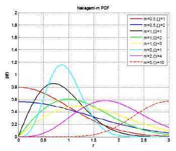
Figure 1. The PDF plot of Nakagami-m distribution.
