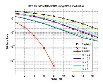
*Figure 5.* BER performance for 2×2 MIMO-OFDM system using BPSK modulation over different channels.
