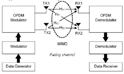
Figure 3. A conventional 2×2 MIMO-OFDM system over Nakagami-m fading channel.
