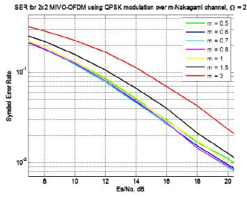
*Figure 6.* SER performance for  $2 \times 2$  MIMO-OFDM using QPSK modulation over Nakagami-*m* fading channel,  $\Omega = 2$ .
