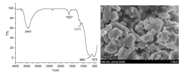
Figure 6. FTIR spectrum and SEM image of spinel MgAl<sub>2</sub>O<sub>4</sub>.
