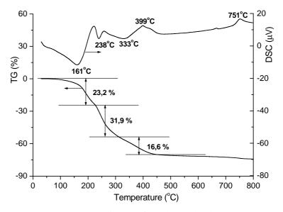
Figure 3. TG-DSC diagram of metals-starch gel precursor.
