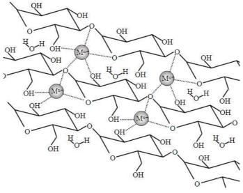
Figure 5. The structure of metals-starch gel precursor [9].
