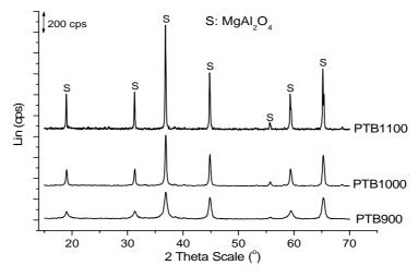
Figure 4. XRD diagram of spinel MgAl<sub>2</sub>O<sub>4</sub>.
