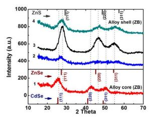
Figure 3 . XRD patterns of the alloy nanocrystals QD samples, with the same shell thickness: from bottom to top: (1)  $Cd_{0.4}Zn_{0.6}Se$  core (2)  $Cd_{0.4}Zn_{0.6}Se/ZnSe_{0.2}S_{0.8}$ . 4ML (3)  $Cd_{0.4}Zn_{0.6}Se/ZnSe_{0.5}S_{0.5}$ . 4ML and (4)  $Cd_{0.4}Zn_{0.6}Se/ZnSe_{0.6}S_{0.4}$ .4ML.
