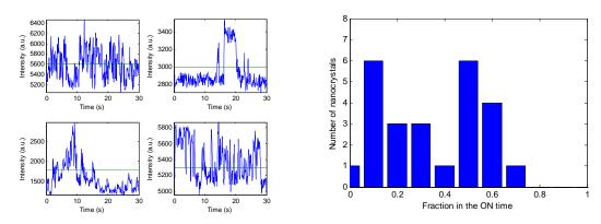
Figure 9. Left: Intensity time traces of four different nanocrystals, measured by CCD camera with a 100 ms resolution for sample Cd<sub>0.39</sub>Zn<sub>0.61</sub>Se/ZnS 4ML (N8-4-12) (the threshold between ON and OFF states is plotted in green). In right: Histogram of the fraction of time spent by each nanocrystal in the ON state for the same sample.
