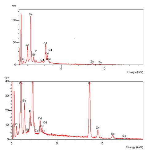
Figure 2. EDX spectra of  $Cd_{0.4}Zn_{0.6}Se$  quantum dots (on top) and  $Cd_{0.4}Zn_{0.6}Se/ZnS$  4ML (below)
