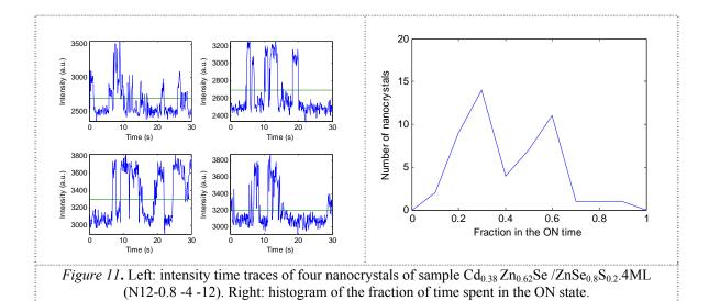
To carry out in a similar way, we measured the PL blinking of the other samples. Figures 10 and 11 present the results of PL blinking of the samples  $Cd_{0.38} Zn_{0.62}Se$  (N12-0-12) and  $Cd_{0.38} Zn_{0.62}Se$  /ZnSe<sub>0.8</sub>S<sub>0.2</sub>. 4ML.
