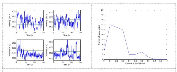
Figure 10. Left: intensity time traces of four nanocrystals of sample Cd<sub>0.38</sub> Zn<sub>0.62</sub>Se (N12-0-12). Right: histogram of the fraction of time spent in the ON state.
