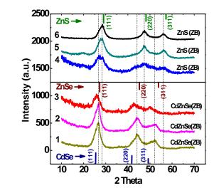
Figure 1. XRD patterns of the alloy nanocrystals QD samples on Si wafer substrates, with different shell thickness: from bottom to top: (1)  $Cd_{0.4}Zn_{0.6}Se$  (reaction time-28 min), (2)  $Cd_{0.4}Zn_{0.6}Se$  (reaction time-20 min), (3) CdZnSe (240 °C, 18 min), (4)  $Cd_{0.4}Zn_{0.6}Se/ZnS$  2ML, (5)  $Cd_{0.4}Zn_{0.6}Se/ZnS$  4ML,and (6)  $Cd_{0.4}Zn_{0.6}Se/ZnS$  6ML.
