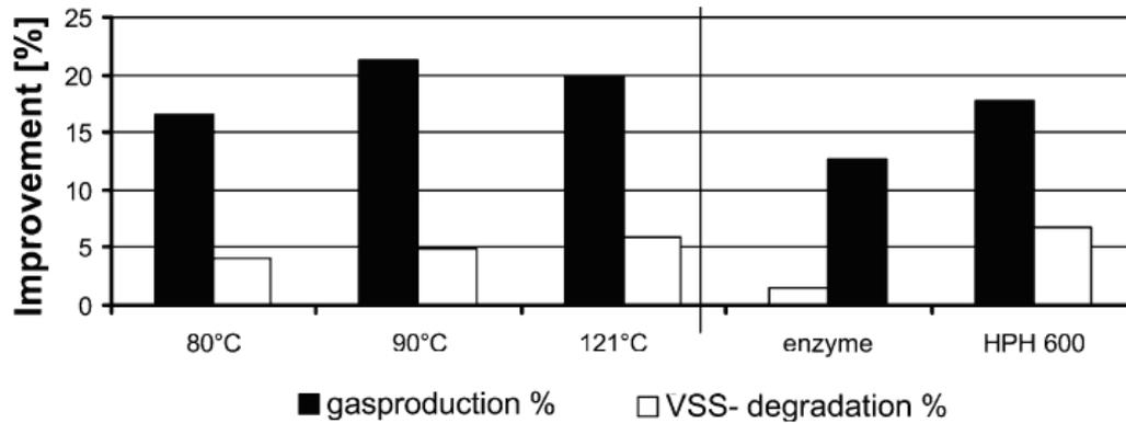
Figure 11. Improvement in anaerobic degradation compared to the control reactor [60].
