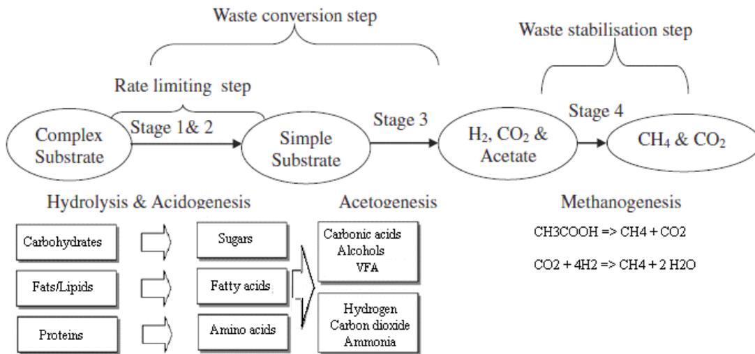
Figure 5. The main stages in anaerobic digestion process [15].
