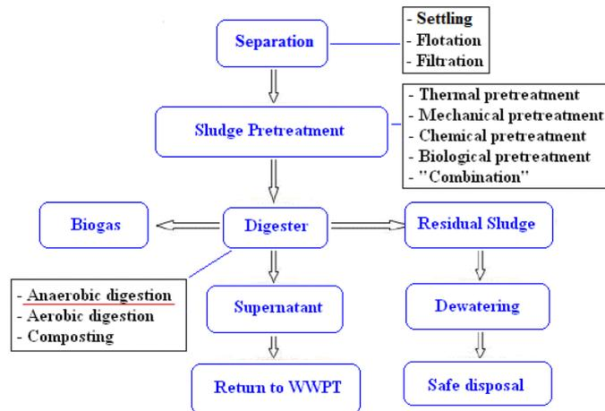
Figure 1. Process flowchart of sludge processing steps [1].
