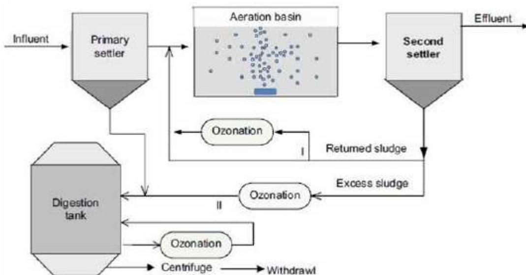
Figure 8. Application of ozonation for sludge disintegration [119].
