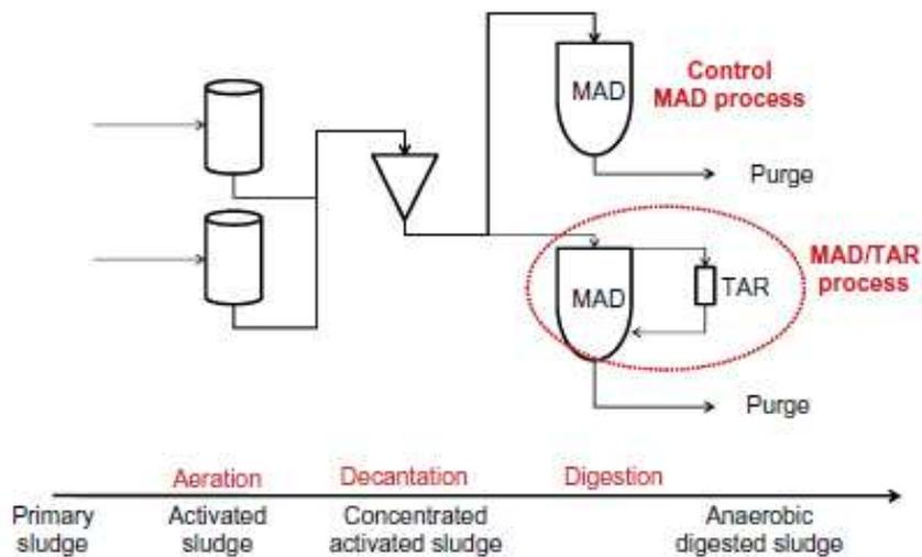
Figure 4. Aerobic hyper-thermophilic co-treatment [12].
