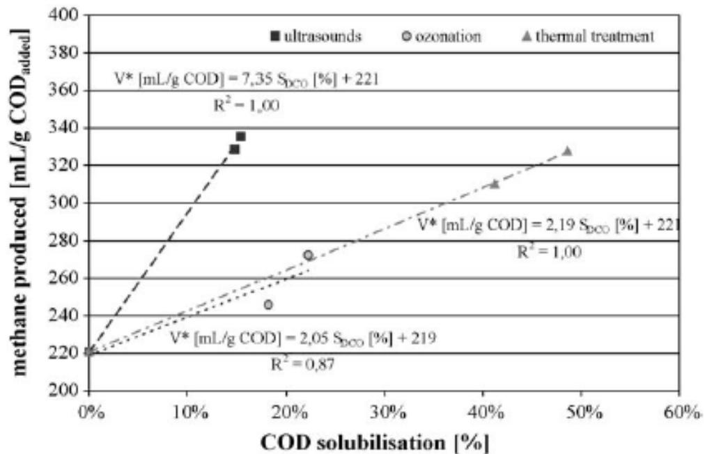
Figure 9. Methane production vs. SCOD for different pretreatment techniques [139].
