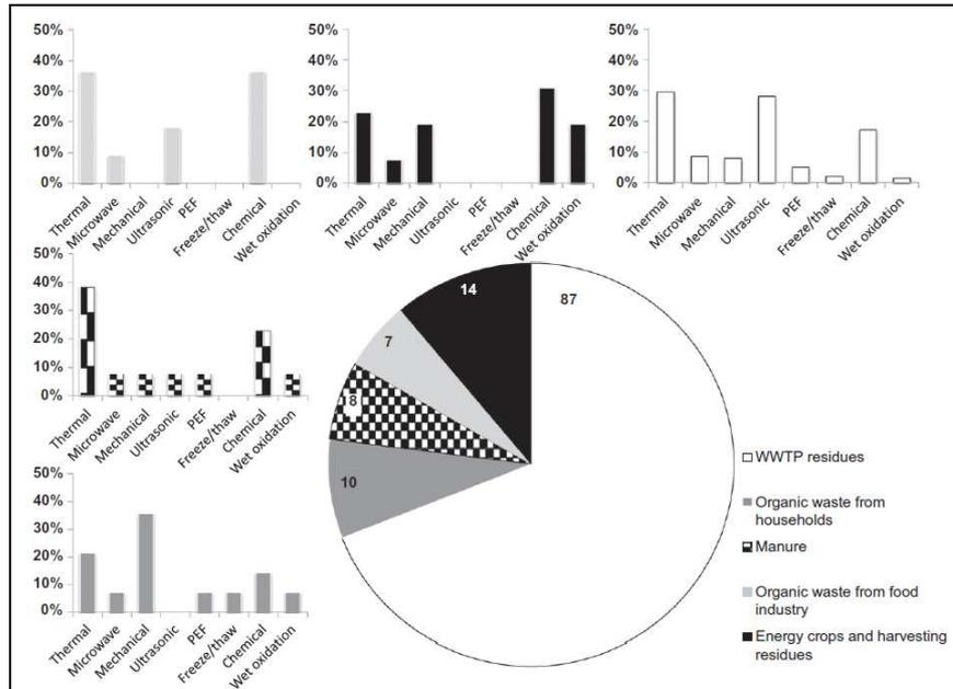
Figure 2. Collection of pretreatment techniques and sludge types [2]. The pie-chart corresponds to the number of times each sludge type occurs in combination with a pretreatment. The bar-charts present the distribution among the different pretreatments for each type of sludge.
