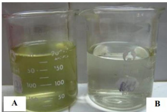
Figure 8. Comparison of wastewater color of pre-treatment (A) and post-treatment (B) wastewater.
