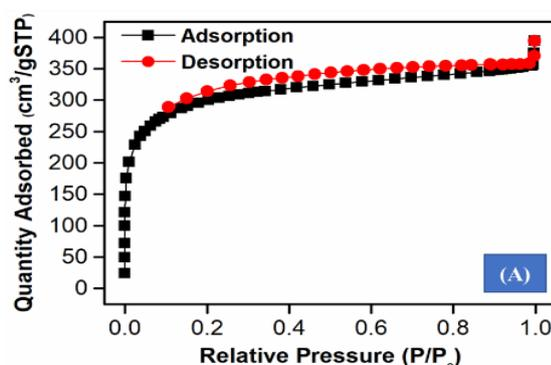
Figure 3. The N<sub>2</sub> adsorption/desorption isothermal of AC from sugarcane bagasse.
