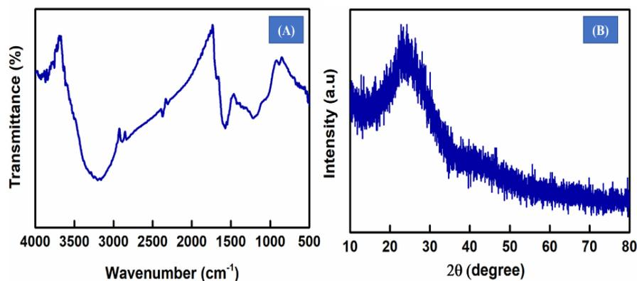
Figure 2. FT-IR spectra (A) and XRD images (B) of AC from sugarcane bagasse.
