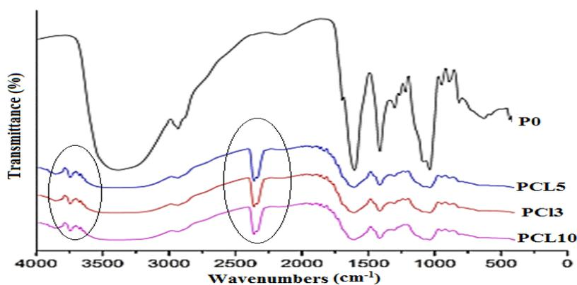
Figure 1. FTIR spectra of P0, PCL3, PCL5, and PCL10 composite films.
