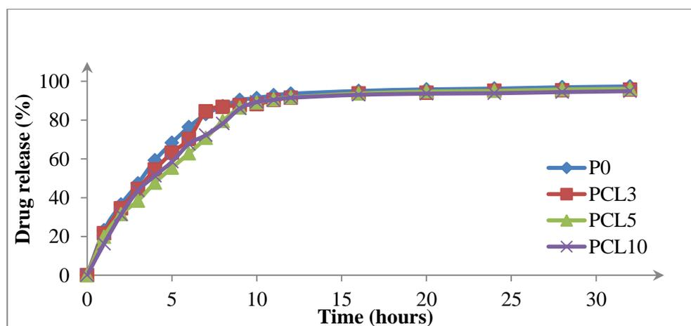
Figure 4. LS release content from P0, PCL3, PCL5 and PCL10 composite films in pH 6.8 phosphate buffer solution.
