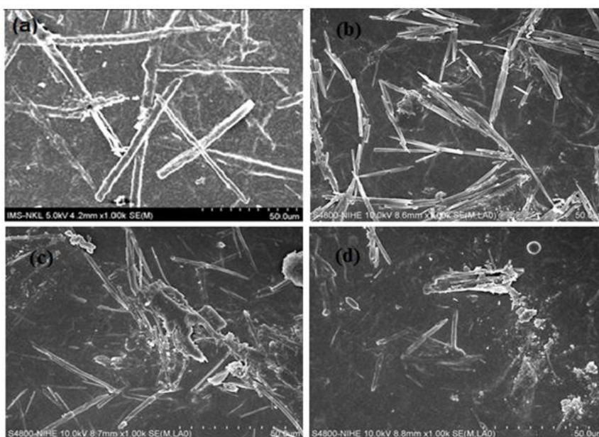
Figure 3. FESEM images of P0 (a), PCL3 (b), PCL5 (c), and PCL10 (d) composite films.
