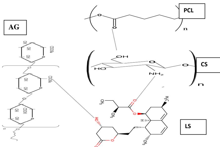
Figure 2. A hypothetical model of hydrogen bonding between AG, CS, PCL, and LS in composite films.
