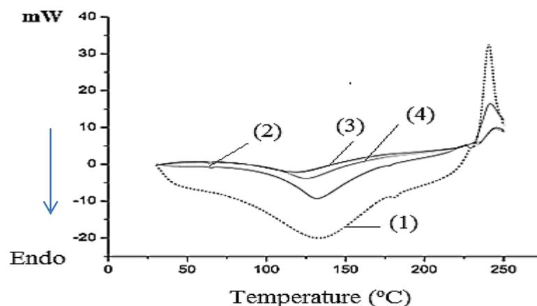
Figure 3. DSC diagrams of P0 (1), PCL3 (2), PCL5 (3) and PCL10 (4) composite films.
