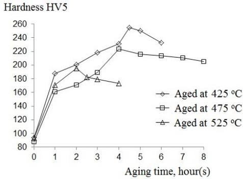
Figure 4. The changes in hardness of specimens after ST + CR 0 % + aging.
