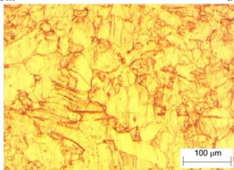
Figure 14. Microstructure of alloy specimen after aging at 525 °C for 4h with 70 % cold pre-deformation.
