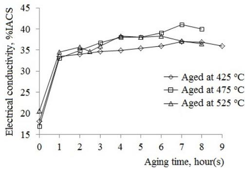
Figure 10. The changes in electrical conductivity of specimens after ST + CR 45 % + aging.
