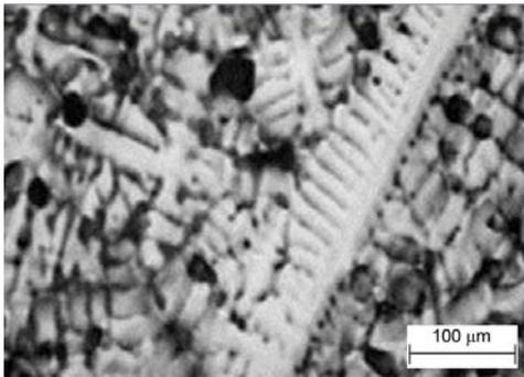
Figure 1. As-cast microstructure of Cu-2.8Ni-1.0Si alloy.
