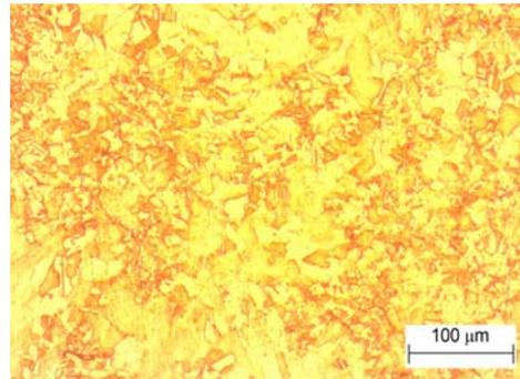
Figure 2. Microstructure of Cu-2.8Ni-1.0Si alloy after solution treatment and quenching.
