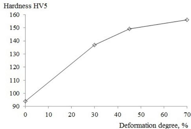
Figure 3. Effect of cold deformation degree on hardness of Cu-2.8Ni-1.0Si supersaturated alloy.
