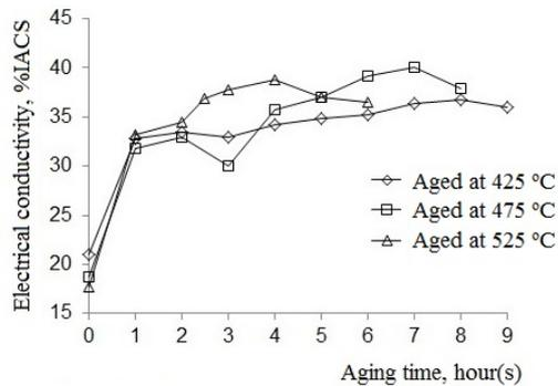
Figure 9. The changes in electrical conductivity of specimens after ST + CR 30 % + aging.
