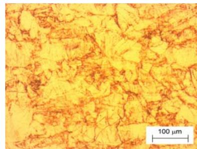
Figure 13. Microstructure of alloy specimen after aging at 475 °C for 6h with 70 % cold pre-deformation.
