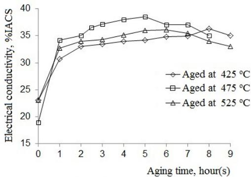
Figure 8. The changes in electrical conductivity of specimens after ST + CR 0 % + aging.
