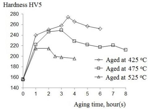
Figure 7. The changes in hardness of specimens after ST + CR 70 % + aging.
