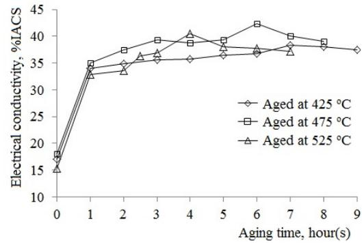
Figure 11. The changes in electrical conductivity of specimens after ST + CR 70 % + aging.
