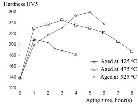
Figure 5. The changes in hardness of specimens after ST + CR 30 % + aging.
