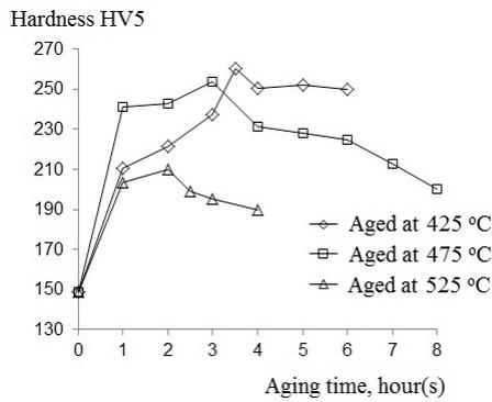
Figure 6. The changes in hardness of specimens after ST + CR 45 % + aging.
