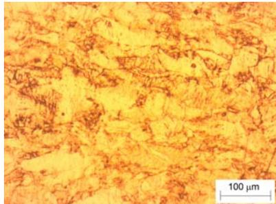
Figure 12. Microstructure of alloy specimen after aging at 425 °C for 8h with 70 % cold pre-deformation.
