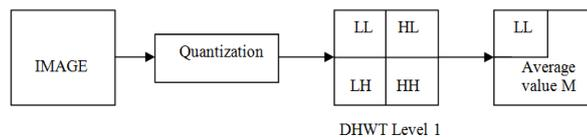
Figure 1. The Scheme of lossy 2D-DHWT level 1
