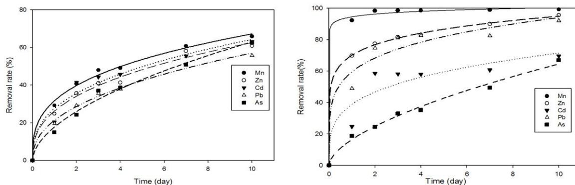
Figure 2. Cumulative removal rates of heavy metals and As in Tank B (left) and C (right).
