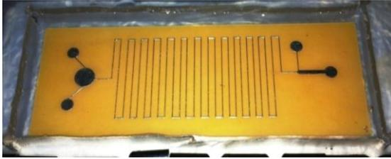
Figure 1. PDMS resin in mould after solidifying.
