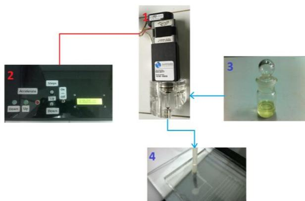
Figure 4. The micro-flow pump connecting the microfluidic chip. 1) The micro-flow pump system with step motor. 2) The control panel. 3) The analyzed solution. 4) The microfluidic chip.
