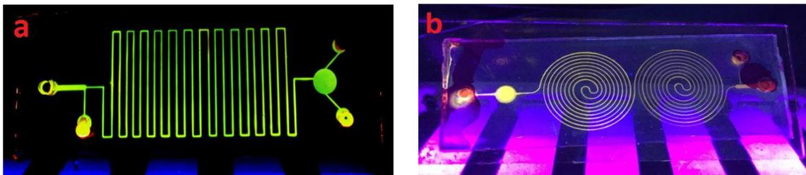
Figure 5. Microfluidic chips of two sets of channel: straight (a) and spiral are radiating under UV light.
