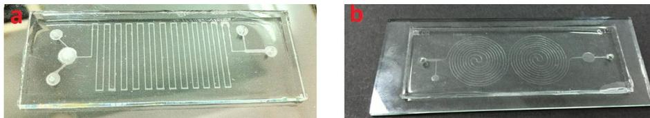
Figure 3. The microfluidic chip with straight (a) and (b) spiral channel after finishing.
