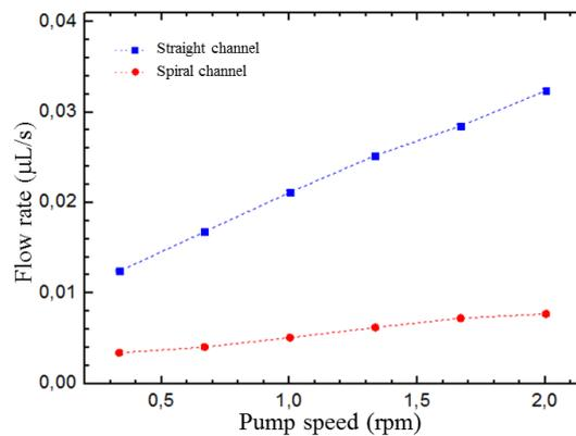
Figure 6. Evolution of flow velocity of two sets of channels: straight and spiral as a function of pump rate.
