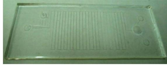
Figure 2. The PDMS surface with straight pattern of channel after being peeled off from the mould.
