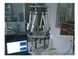
Figure 4: The experimental system (Stewart – Gough Platform)
