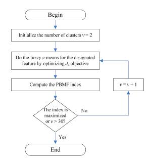
Figure 2: The flow chart of the fuzzy c-means clustering technique together with the PBMF index validation.
