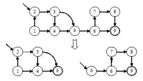
Fig.1. An example of partitioning of an N-ADFA at a bridge state b
