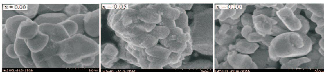
Fig. 2. SEM images of Sm doped  $\text{ZnWO}_4$  nanopowders
