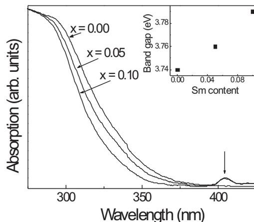
**Fig. 3.** Absorption spectra of Sm doped ZnWO<sub>4</sub> nanopowders
