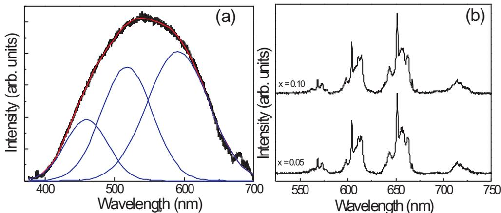
**Fig. 5.** (a) PL spectra of the  $ZnWO_4$  synthesized by the hydro thermal method for 8 h (the solid lines are fitting results by using Gauss distribution); (b) Emission spectra of the  $Sm^{3+}$  doped  $ZnWO_4$  at room temperature
