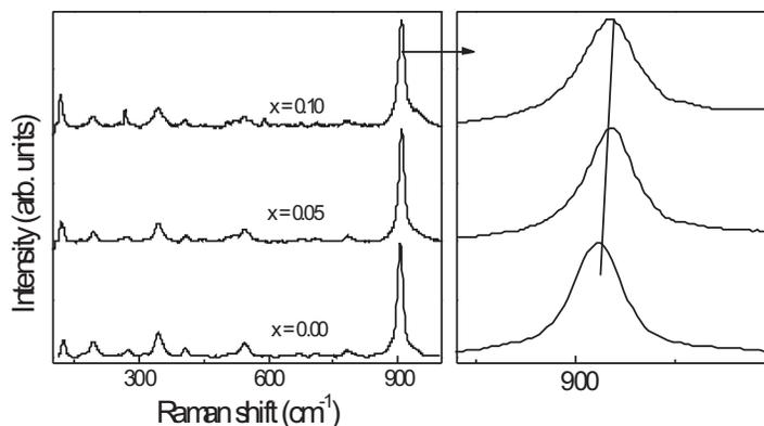
**Fig. 4.** Raman spectra of Sm doped ZnWO<sub>4</sub> nanopowders. The right one is the enlarged peak of 900 cm<sup>-1</sup>.
