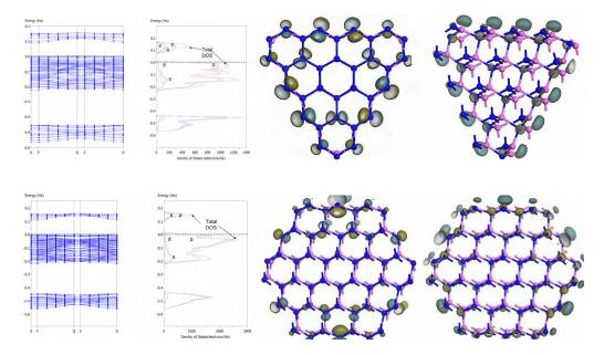
Fig. 5. (from the left to right) The band structures for relaxed triangular (T-4) and hexagonal (H-3) nanowire. The total DOS as well as PDOS of H-3 and T-4 are showing next to the bandstructures. The (HOMO) and (LUMO) states of the wire.
