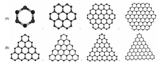
Fig. 1. (Color online) AlN nanowires in [0001] direction with (A) hexagonal and (B) triangular shaped cross sections, viewed along the wire direction. Nitrogen and Aluminum atoms are indicated by the light (purple) and dark (blue) spheres, respectively.
