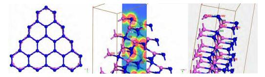
**Fig. 3.** (Color online) AlN Nanowires in [0001] direction with one representative triangular (T-4) fully optimized structure with cross section view and a view along the wire direction. See Fig. 2 for details.
