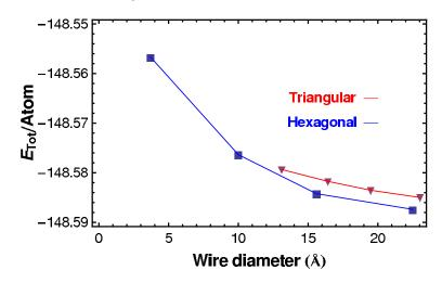
**Fig. 4.** (Color online) Diameter dependence of the cohersive energy for the various type AlN nanowire. The blue line (dark) with filled box is hexagonal and purple (light and dashed) with triangular is triangular wire, respectively.
