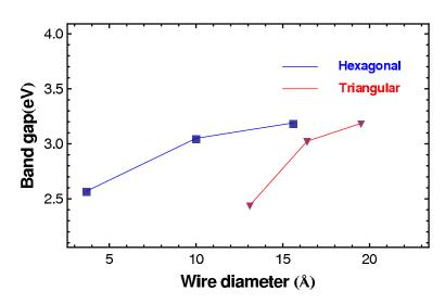
**Fig. 6.** Band gap as a function of nanowire diameter, filled box for hexagonal and triangular for triangular wire , respectively.
