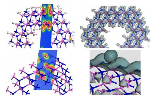
Fig. 8. ((upper row) Relaxed hexagonal tube-like nanowire terminated by hydrogen atom (Al-H) and (N-H) from left to right with i) Mulliken charge labeled in atom site and bond length label in selective bonds and cut plane showing charge redistribution around the bond; (ii) isosurface with charge density with selective Mulliken charge and bond length; (lower row) Relaxed hexagonal tube-like nanowire terminated by hydrogen molecule (Al-H<sub>2</sub>) with similar detail as in the upper row.
