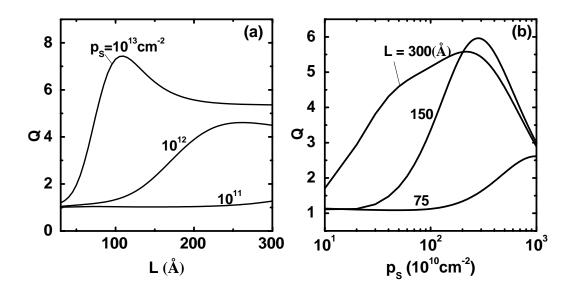
Fig. 1. Mobility enhancement factor Q for the *p*-type square QW with a fixed correlation length  $\Lambda = 75$  Å vs (a) the well width L for various sheet hole densities  $p_s$  given on lines, and (b) the hole density  $p_s$  for various well widths L given on lines.
