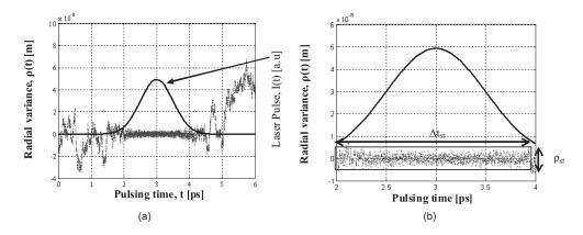
**Fig. 2.** (a) Radial variance of glass particle in water during pulse time. (b) The stable space-time pillar created within the interval  $[-\tau, \tau]$ .
