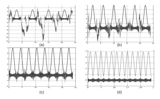
Fig. 6. Stability process of particle in optical tweezer pumped by series of laser pulses with different repetition period. (a):  $T = 6\tau$ , n = 4; (b):  $T = 4\tau$ , n = 6; (c):  $T = 3\tau$ , n = 8; (d):  $T = 2\tau$ , n = 12. Note: Vertical unit [nm]; Horizontal unit  $[\tau]$ .
