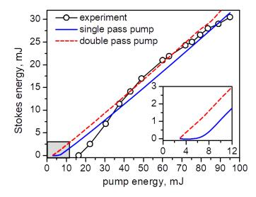
**Fig. 3.** Experimentally measured (hollow dots) and numerically calculated for singlepass (blue solid line) and double- pass (red dashed line) pump configurations Stokes energy as a function of the pump energy.
