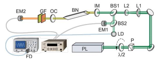
**Fig. 1.** Principal scheme of the experimental setup: PL: frequency-doubled Nd:YAG pump laser;  $\lambda/2$ : half-wave plate at the 532 nm wavelength; P: polarizer; L1,2: positive and negative lenses of the pump beam compressor; BS1,2: beam splitters; IM: input mirror of the Raman cavity; BN: barium nitrate crystal; OC: output coupler of the Raman cavity; GF: color glass filters; LD: light diffuser; EM1,2: sensors of the energy meter; FD: fast photodetector.
