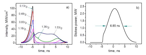
**Fig. 5.** The double-pass pump configuration: (a) intensity profiles of the depleted pump pulse for different displacement from the beam optical axis; (b) power profile of the corresponding Stokes pulse.
