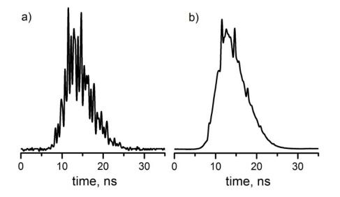
**Fig. 2.** Typical single-shot (a) and cumulative over  $10^3$  laser shots (b) oscilloscope traces of the pump pulses.
