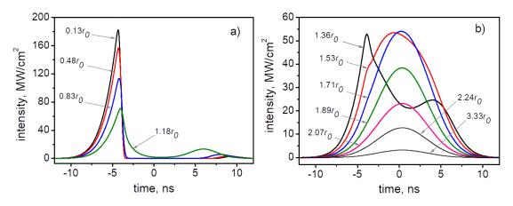
**Fig. 4.** The single-pass pump configuration: intensity versus time profiles of the depleted pump pulse issued from numerical calculations for different displacements from the beam optical axis.
